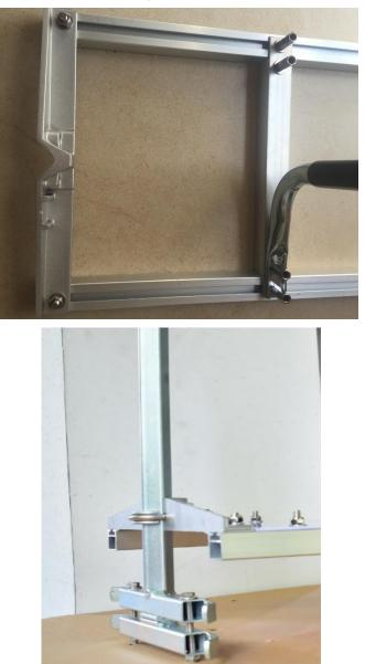
With the end post assembly attached to the frame bracket and long rails, adjust to desired cutting thickness (minimum 3 inches) and tighten nuts around U-Bolt.
