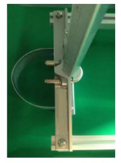
With the guard assembly attached to the frame bracket and long rails, adjust to desired cutting thickness (minimum 3 inches) and tighten nuts around U-Bolt.
