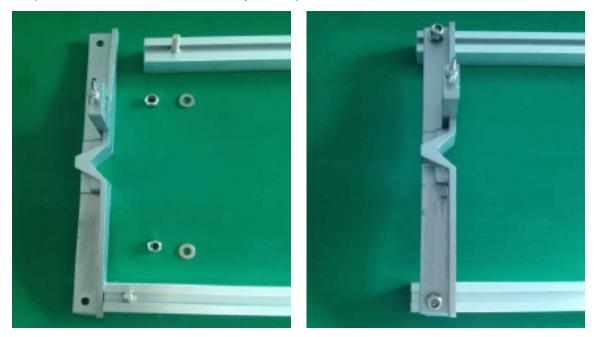
7. Attach chain guard assembly to the frame bracket (#6) using U-Bolt (#9)m U-Bolt Adaptor/Clamp (#10), washers (#11), and long hex nuts (#2).
